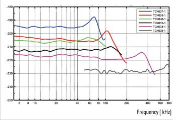
Transmitting Voltage Response Teledyne RESON Reference Hydrophone [ dB re.  $1V/\mu Pa @ 1m$  ]
